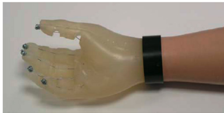
Figure 16: The compliant hand from University of Pisa, as presented in [17]
