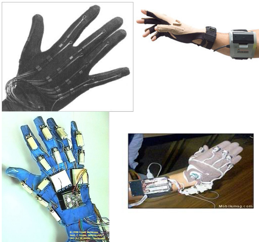
Figure 2: Different data-glove images, obtained from the manufacturer's web pages. From left to right: upper row, VPL dataglove and Virtex cyberglove. Lower row, TUB SGlove and GWU AcceleGlove
