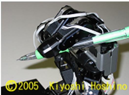
Figure 13: Anthropomorphic hand with pinching capabilities [41]
