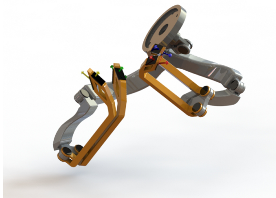
Fig. 13. Final hand design with fingertips reaching task positions 1, 2 and 3. The task positions are indicated with reference frames.
