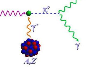
$$\frac{d\sigma_P}{d\Omega} = \Gamma_{(\pi^0 \to \gamma\gamma)} \frac{8\alpha_{em}Z^2}{m^3} \frac{\beta^3 E^4}{Q^4} |\tilde{F}_{em}(Q)|^2 \sin^2\theta_{\pi}$$
