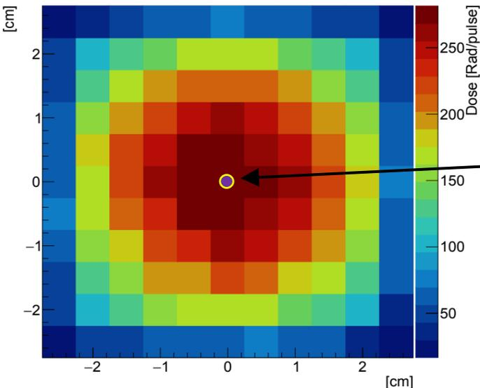
Simulated beam calibrated with beamspot measurements at 3 distances
