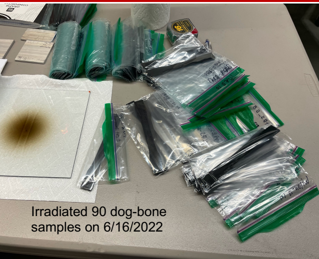
3D-printed carbon-fiber embedded nylon ASTM-D638 dog-bones
