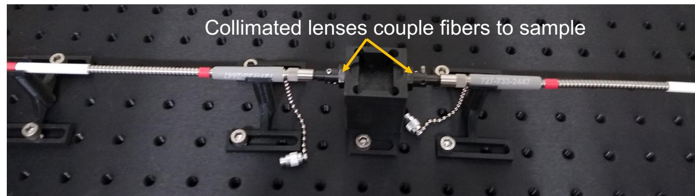
New 3D-printed sample holders – can fabricate for any sample geometry
