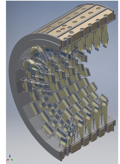
The two detector halves separate to facilitate installation of the detector sector modules.
