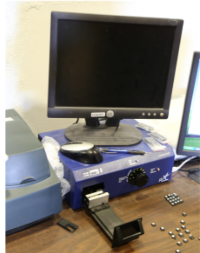
Optically Stimulated Luminescence (OSL) dosimeter (~ 7 mm by 7 mm square)
