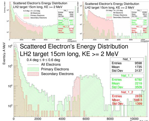
Results from new G4 SAM simulation run for 15 cm LH<sub>2</sub> target and 11 GeV beam with 2 by 2 mm<sup>2</sup> raster: Rate per SAM per  $\mu$ A is  $\sim$ 80MHz
