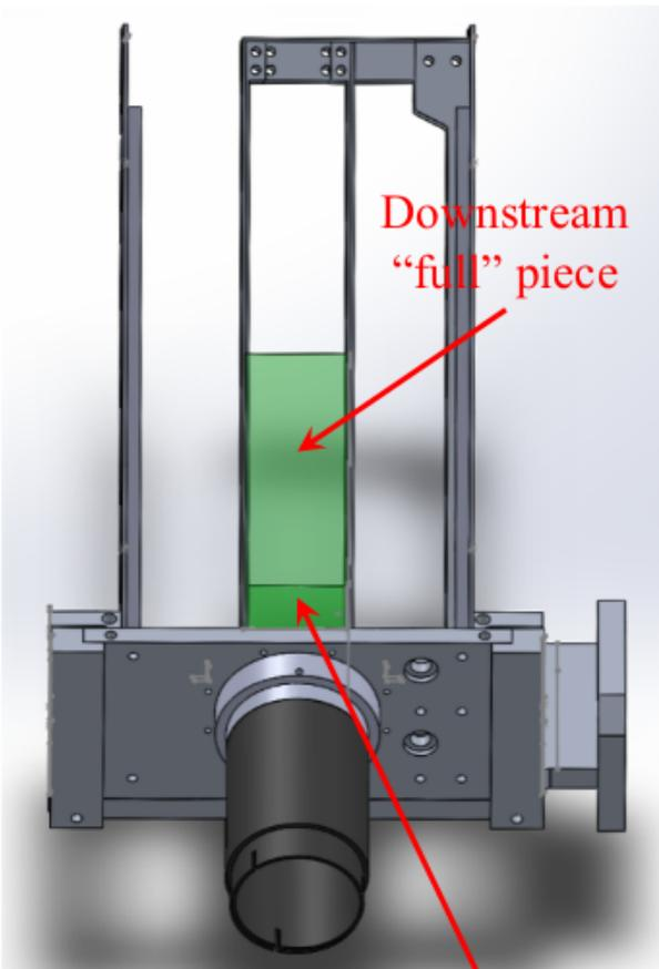
Beam's view. Note "stubby" quartz installed upstream, "full" quartz downstream – for illustrative purposes
