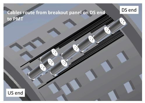
All cables can be disconnected from custom PP to facilitate segment install/de-install 8
