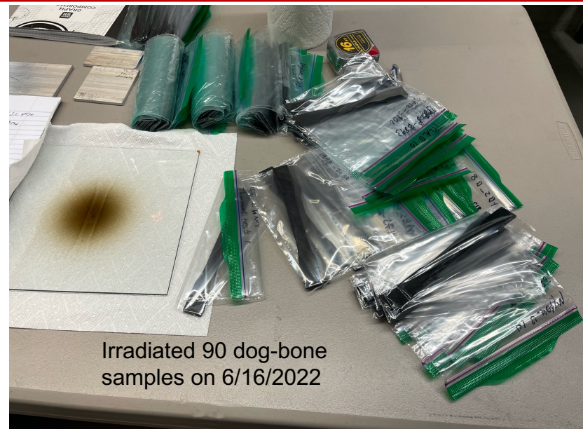
3D-printed carbon-fiber embedded nylon ASTM-D638 dog-bones
