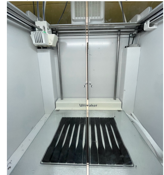
3D-printed ASTM-D638 dog-bones
