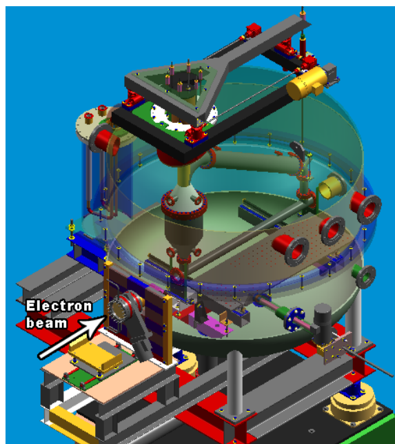
Figure 10: A CAD drawing of the SLAC E18 target chamber. The target loop is remotely movable 6 in in the vertical direction. A table containing optics targets can be moved in and out horizontally.
