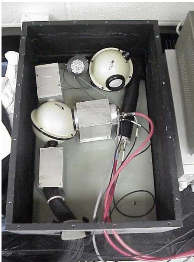
Figure 25: The prototype light monitoring system.
