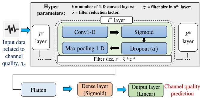
Fig. 2: Proposed CNN-based training and inference model.
