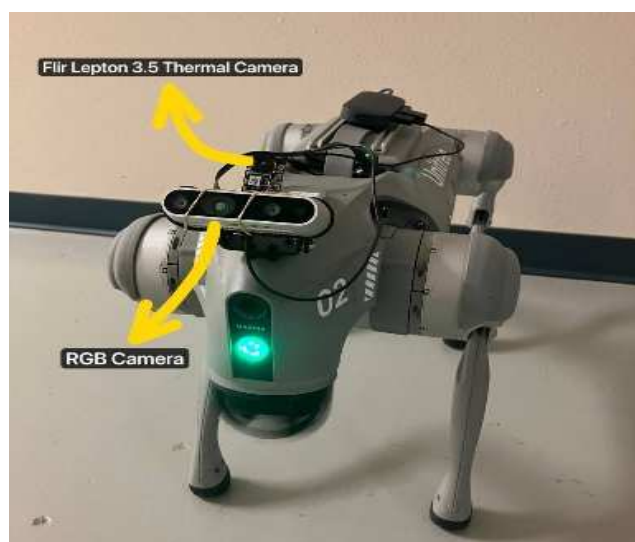
Fig. 3. RGB and Thermal Camera Mounted on the GO2 Edu Dog Robot
