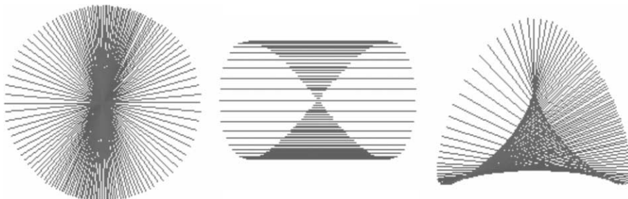
Fig. 2. The cylindroid as viewed first from the top along the central axis, then from the side and finally, from an angle.
